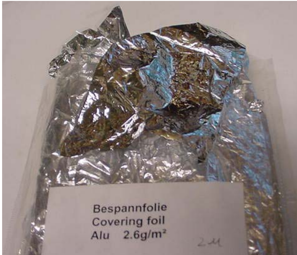
Figure 16: Mylar film, 2 microns thick.
