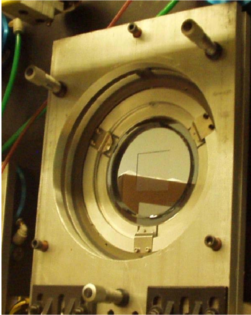
Figure 15: Silicon carbide mask mounted in silicon wafer.
