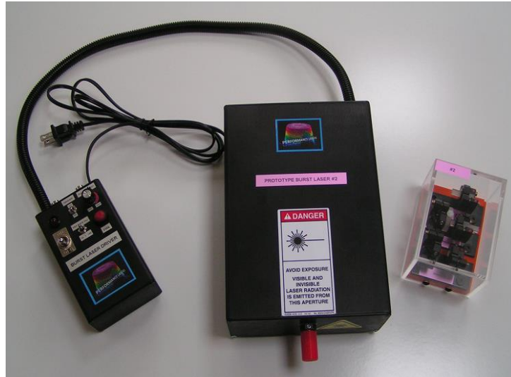
Figure 45 – Complete laser system (laser module in center, laser driver on left, and wavelength converters on right)
