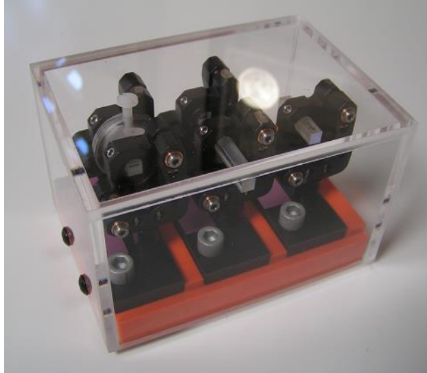
Figure 21 – Dust proof storage enclosure for the various wavelength converters
