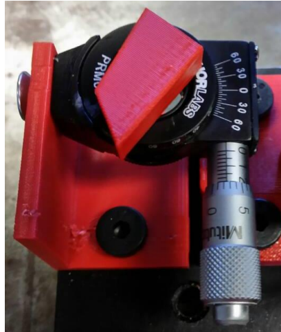
Figure 23 – 3D printed model of PB rotating mount
